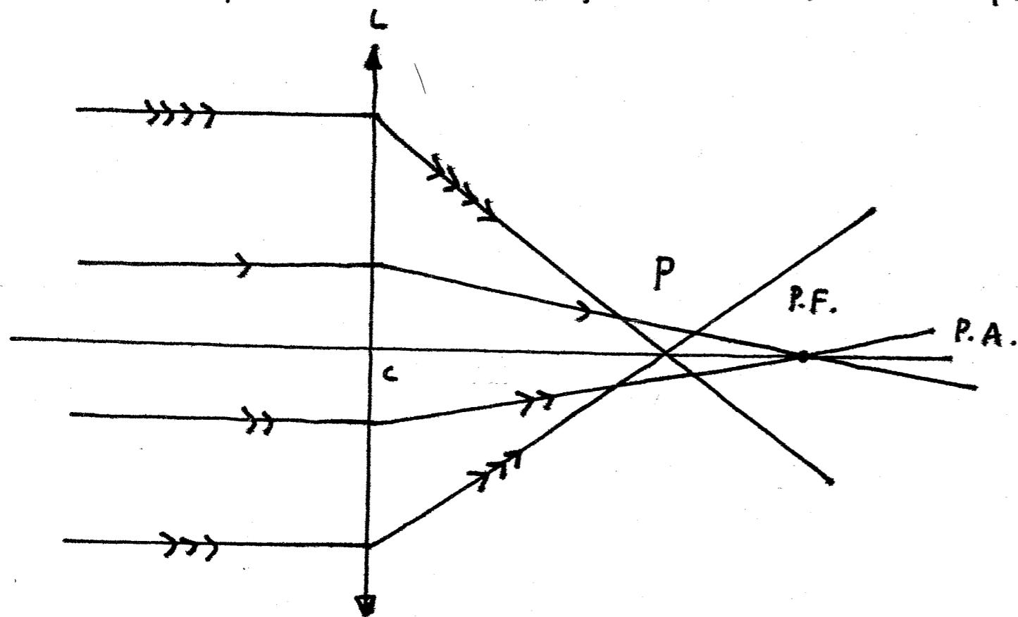
The distance between P and the P.F. is called the longitudinal spherical aberration. Clearly, there will be no sharp image point. A stop, reducing the aperture of the lens to a small central portion, will improve definition — with a consequent reduction in image brightness.
