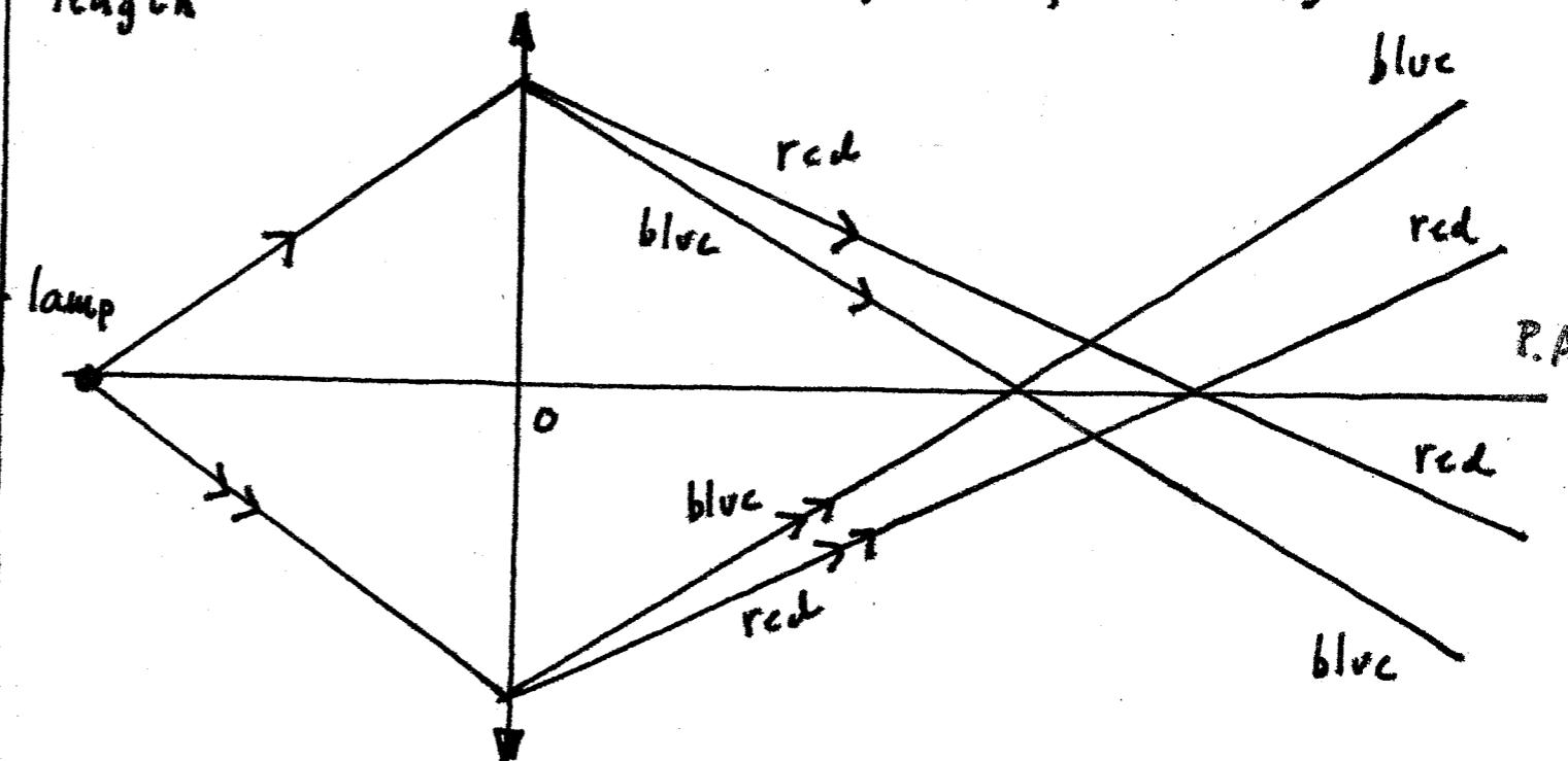
An ordinary lens used to produce a real image of a small bulb, demonstrates chromatic aberration. A screen moved outwards from the lens produces a patch of light orange-red on the outside until the blurred image is reached. Beyond this point, the outside will be blue. An achromatic doublet reduces, but does not eliminate, the problem.
