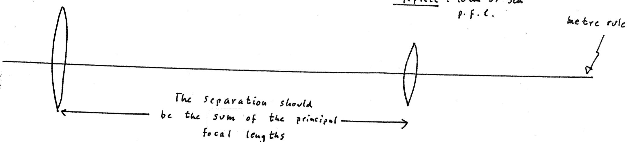
Fix the two convex lenses onto the rule, with plasticine, so that the distance between them is as specified above. Look at distant objects through the arrangement, and verify that it does act as a telescope. The image can be rendered "sharper" by attaching, with plasticine, a circular "stop" of paper.
