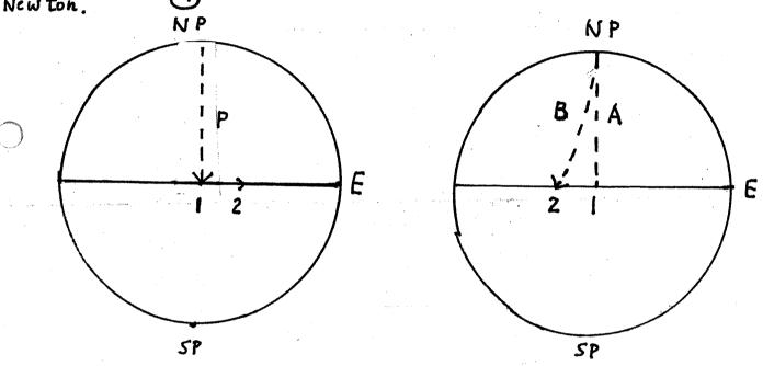
Consider a projectile launched from the North pole, to impact at the Equator. On a non-rotating Earth, the projectile would flow a single meridian of longitude during its entire flight. On a rotating Earth, the target moves Eastward at 0.46kms, and the projectile strikes west of the target. The target moves from 1 to 2, as indicated.
