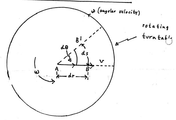
The turntable rotates at the angular velocity, w, Which is the same for all objects on the turntable
